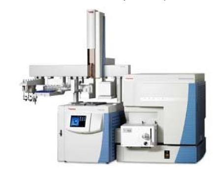
Figure 5: TSQ Quantum XLS Ultra GC-MS/MS System.
